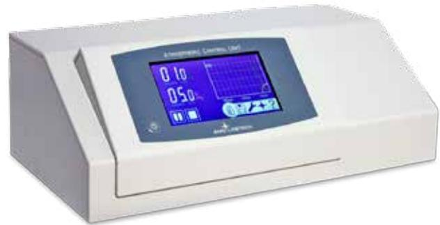
ACU perfectly regulates both O<sub>2</sub> and CO<sub>2</sub> for all cell-based assays.
